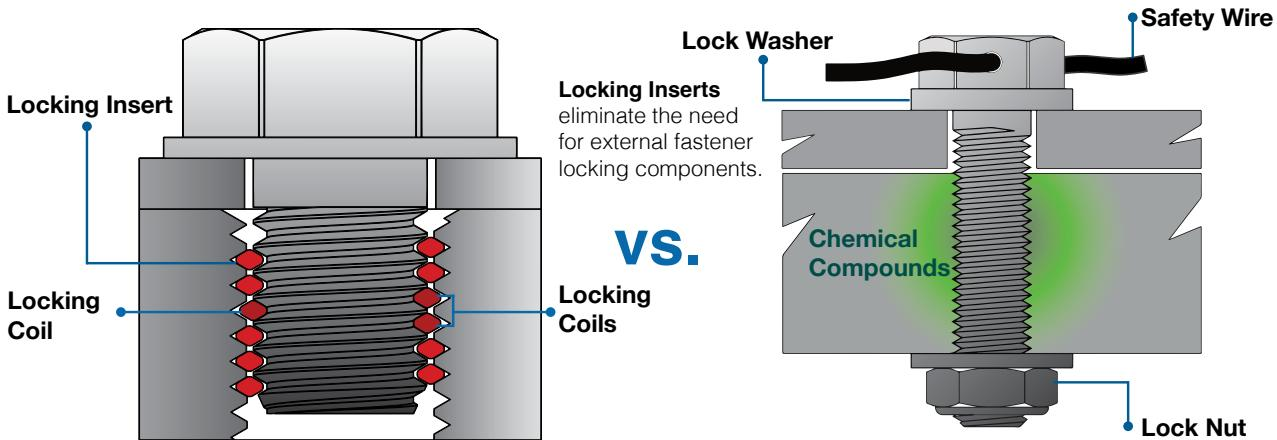
KATO screw locking inserts exert a prevailing torque on male threaded fasteners to prevent loosening due to vibration or impact. Locking inserts eliminate the need for costly and less desirable locking mechanisms. They are excellent in adjusting screw applications by preventing the male fastener from creeping.
