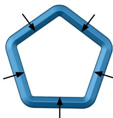
Locking coil segments exert prevailing torque between the thread flanks of the screw, or bolt, to resist loosening.
